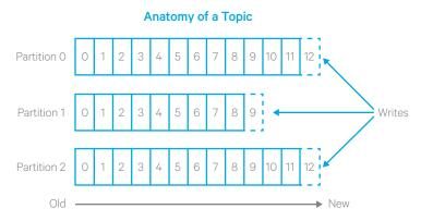
The partitions of a Topic are distributed over the Brokers of the Kafka cluster with each Broker handling data and requests for a share of the partitions. Each partition is *replicated* across a configurable number of Brokers for fault tolerance.
