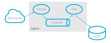
Flume comes with an out-of-the-box library of *Sources* the are optimized for continuous data ingestion from many common sources of data (syslog, http, log4j, etc). Thus, users can perform data ingestion via configuration, without having to write a single line of code.
